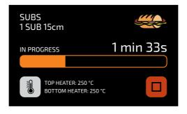
e) If the equipment door is opened, the operation will be paused; once the door is closed again, press the resume the operation.
