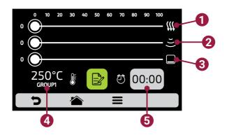
**c)** To change the impinged air speed, microwaves and bottom heating element wattage, just swipe the finger over the bar of each parameter or click on the desired location.
