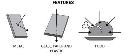
The use of plastic or paper material must respect it's specifications since it must support up to  $280^{\circ}$ C/  $536^{\circ}$ F and being microwavable.
